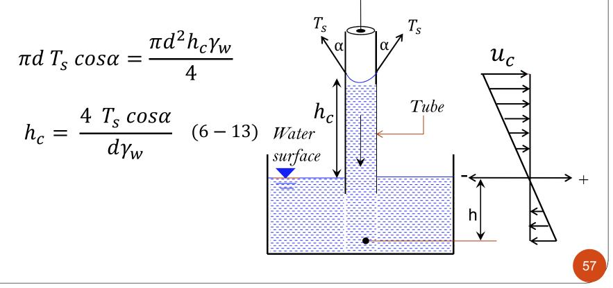
The surface tension  $T_s$  of water at 20°C can be taken as equal to  $75 \times 10^{-8}$  kN per cm. Equation (6–13) can be simplified by assuming  $\alpha = 0$  and by substituting for Ts. Therefore, for the case of water, the capillary height hc can be written as
