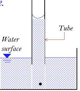
The height of rise of water in the capillary tube can be given by summing the forces in the vertical direction, or  $\uparrow$
