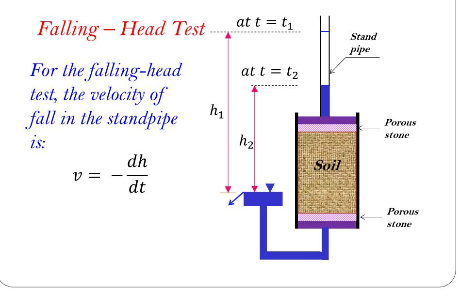
Falling – Head Test  $q_{in} = -a \frac{dh}{dt}$ The flow into the sample is : a = area of standpipe From Darcy's law the flow out is  $q_{out} = k \frac{h}{I} A$ or  $k \frac{h}{L}A = -a \frac{dh}{dt}$  $q_{out} = q_{int}$
