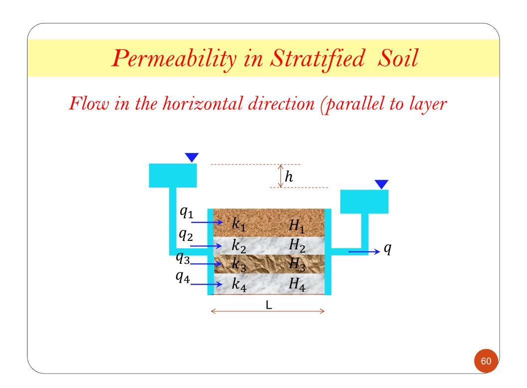
Flow in the horizontal direction (parallel to layer)
