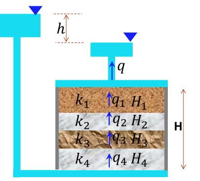
Flow in the vertical direction (perpendicular to layers) The total head loss is the sum of head losses in all layers
